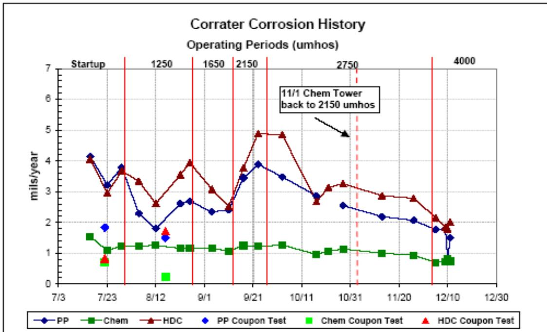
corrosion inhibitor for most of the study. Thus as blowdown volumes decreased, the concentration of corrosion inhibitor increased. While the stated control range was 3-5 mg/l of molybdate, they ranged from 3.0 – 18.5 mg/l concentration with an average of 8.5 mg/l.
